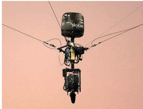
Figure 2 Skycam: a commercialized suspended cable robot
