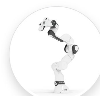
Franka Panda A high-performance, 7-DOF robot, featuring precise torque sensors
